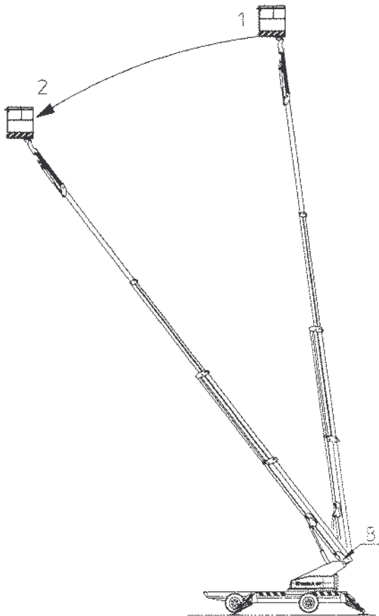
Figure 19-2, Checking the lifting radius
